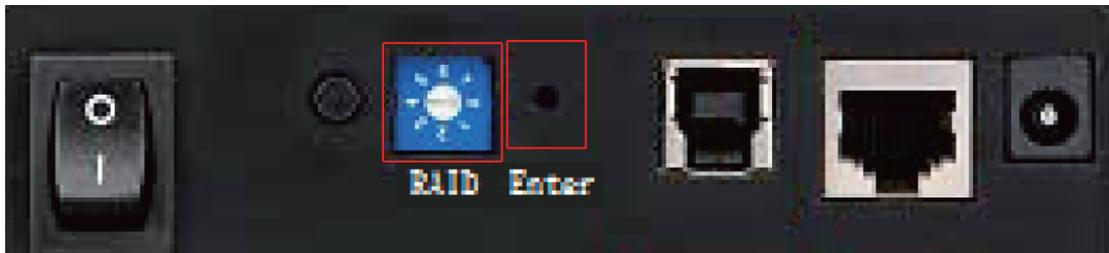
Notes: Please change to single mode before altering any modes of RAID disk array. Otherwise, it cannot be changed. Meanwhile, you should format the HDD by network mode after changing the setting of RAID disk array. After that, it can work in normal.
