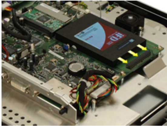
Figure 2-9: IDE HDD Installation
