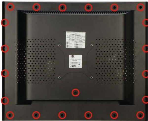
Figure 2-4: iSignager LCD-19 Back Cover Retention Screws
