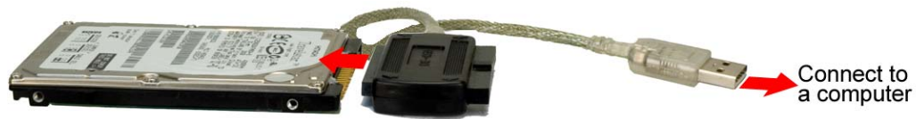
Figure 2-1: Format the HDD via IDE-USB Cable
