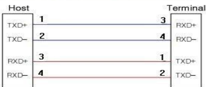
<RS422 Point to Point Networking>
