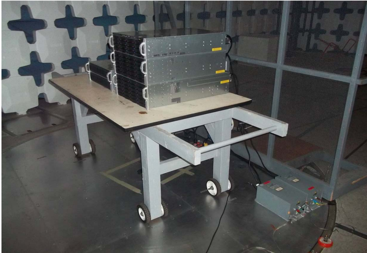
Test Configuration Photograph #1 (Conducted Emissions - Power Port)
