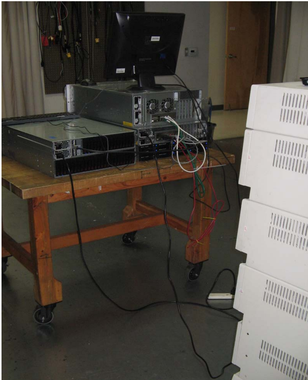
Test Configuration Photograph #2 (Surge, EN 61000-4-5)
