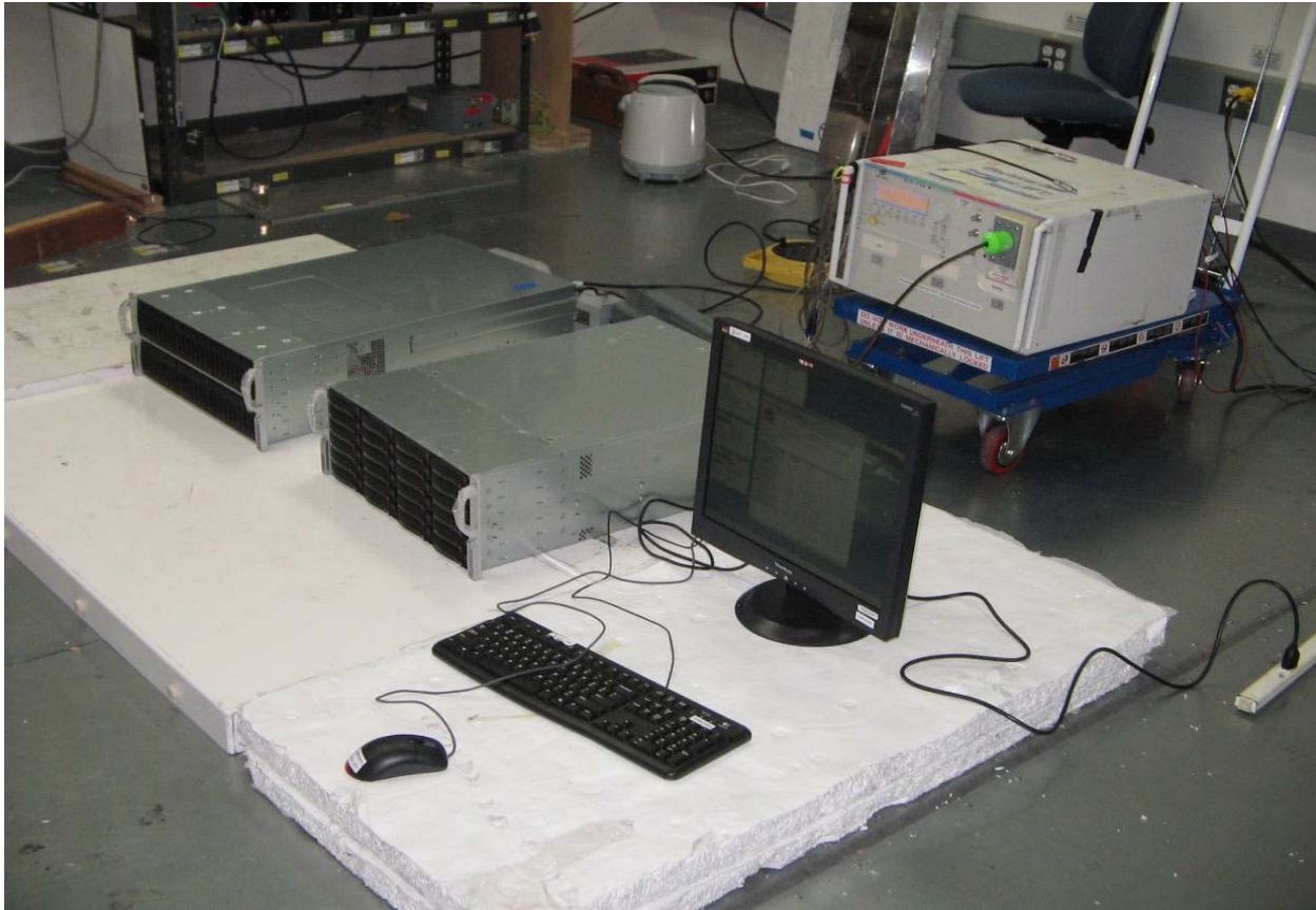
Test Configuration Photograph #1 (Electrical Fast Transient/Burst, EN 61000-4-4) Single sided 4U
