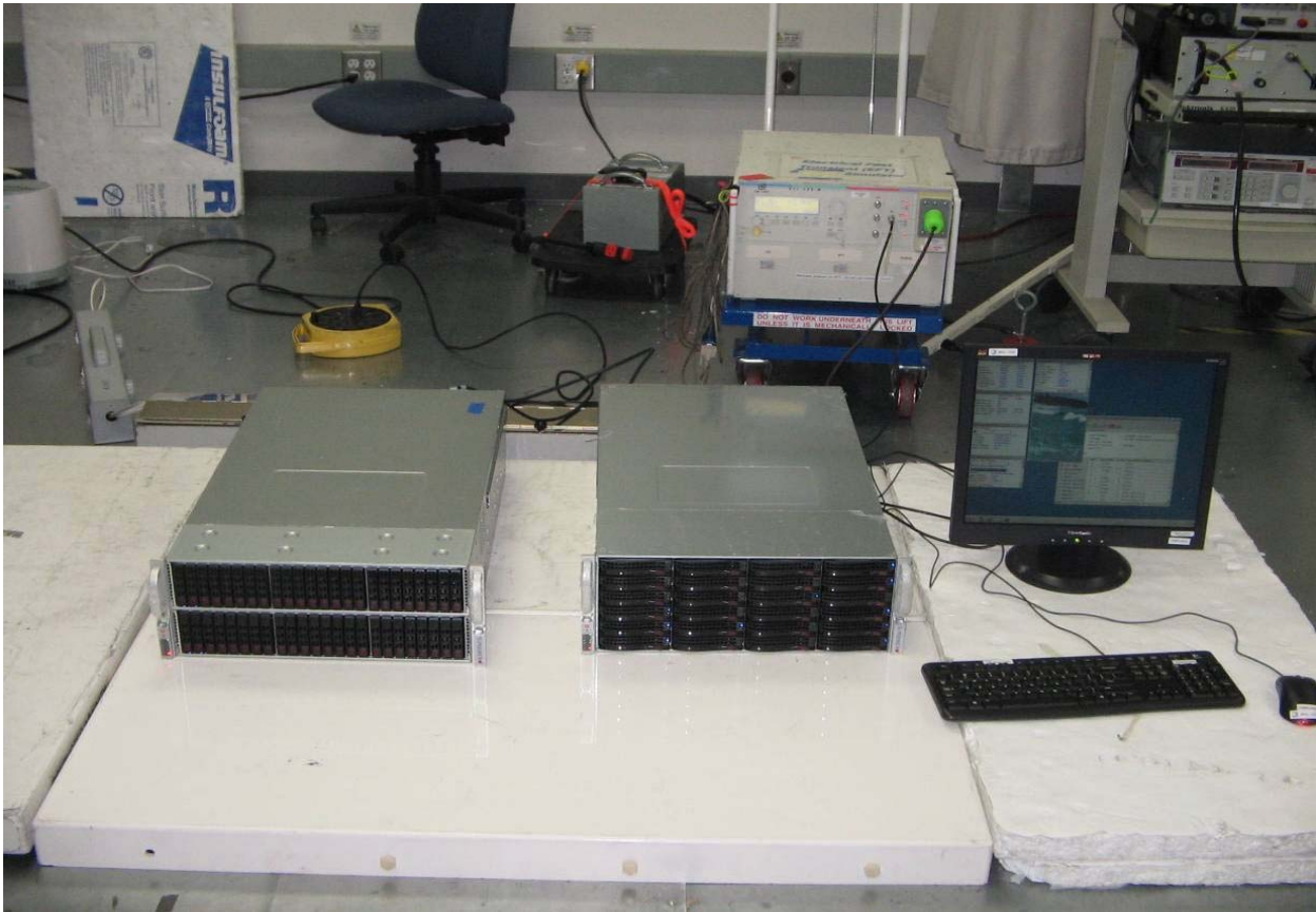
Test Configuration Photograph #1 (Electrical Fast Transient/Burst, EN 61000-4-4) Double sided 4U
