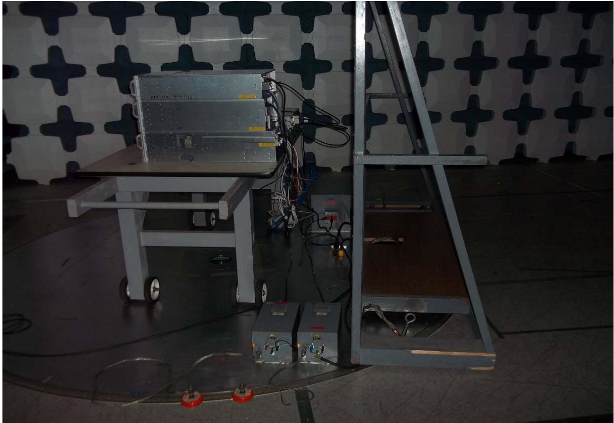
Test Configuration Photograph #2 (Conducted Emissions - Power Port)
