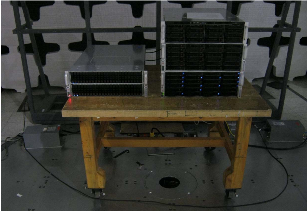
Test Configuration Photograph #1 (Conducted Emissions - Signal Ports)
