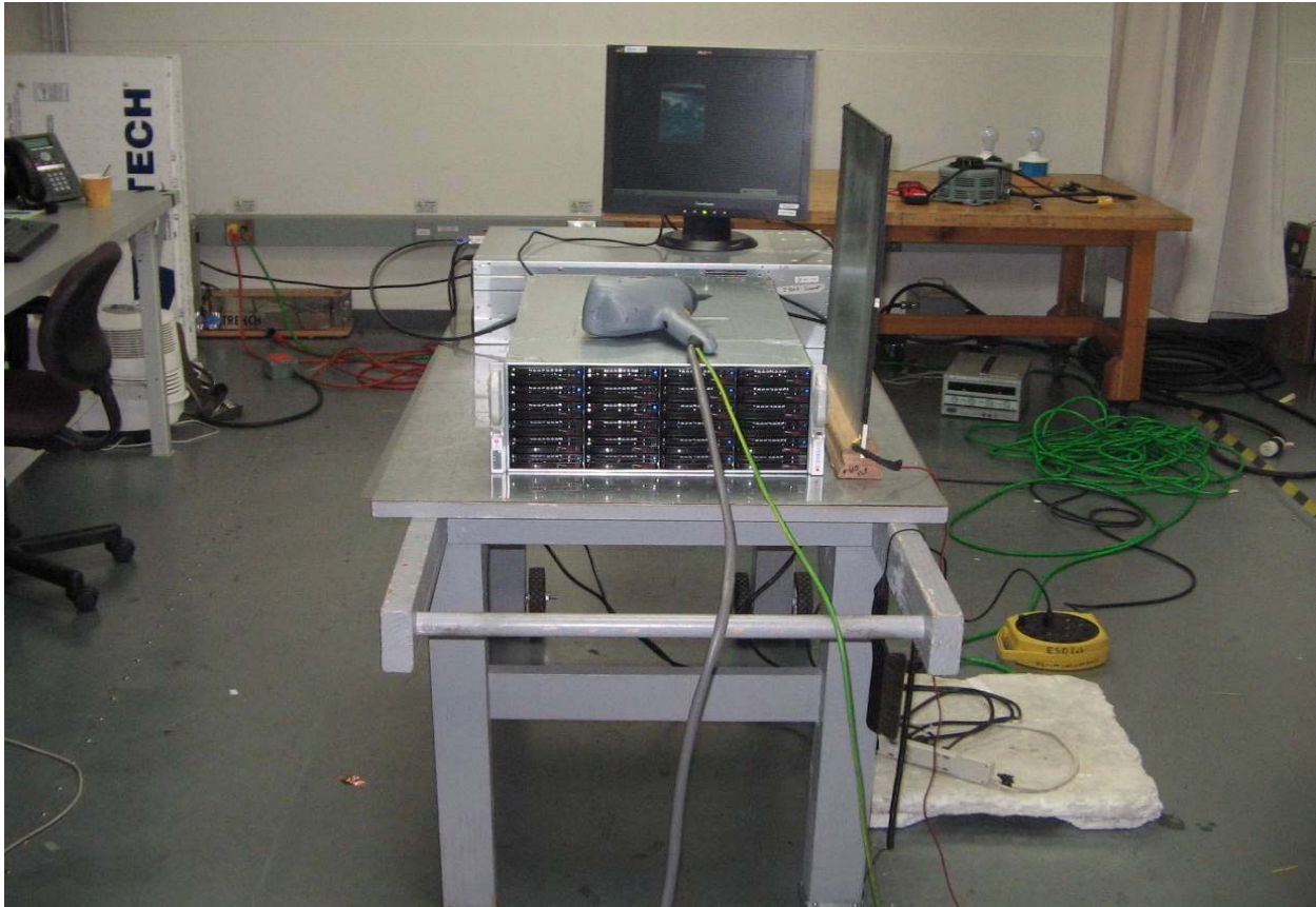
Test Configuration Photograph #1 (Electrostatic Discharge, EN 61000-4-2)
