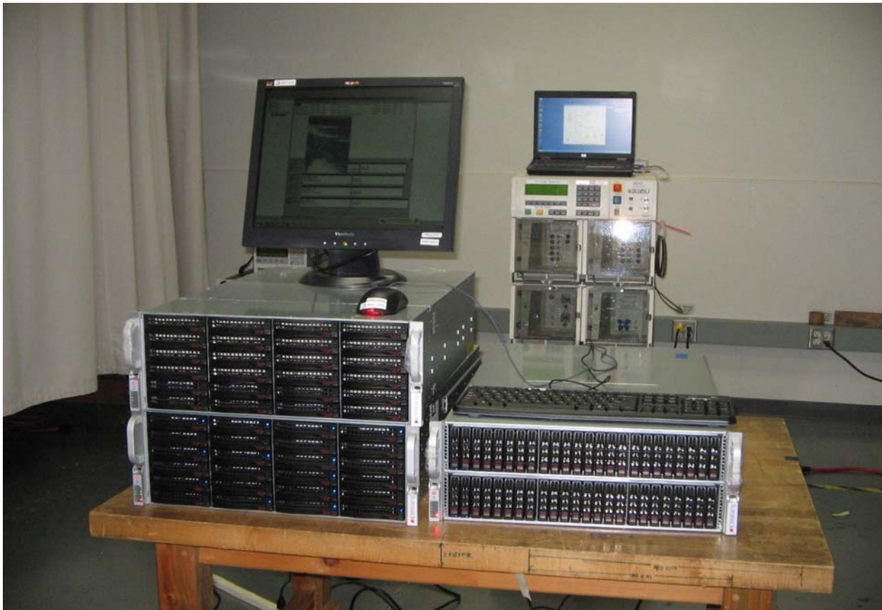
Test Configuration Photograph #1 (Surge, EN 61000-4-5)
