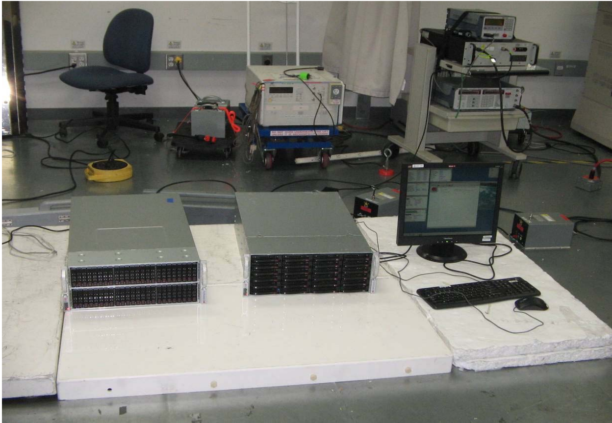
Test Configuration Photograph #1 (Conducted Immunity, EN 61000-4-6) Single sided 4U
