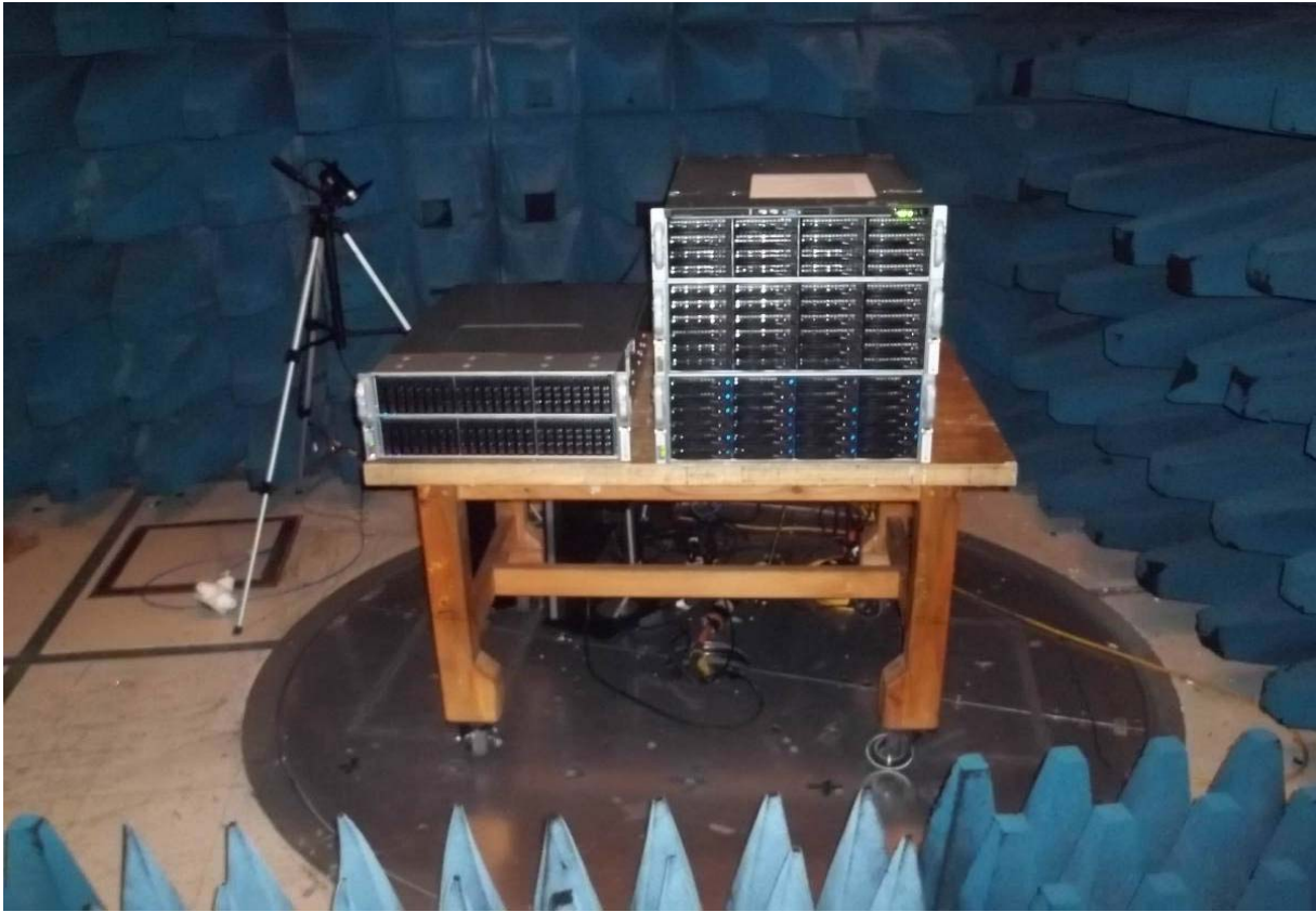
Test Configuration Photograph #1 (Radiated Immunity, EN 61000-4-3)
