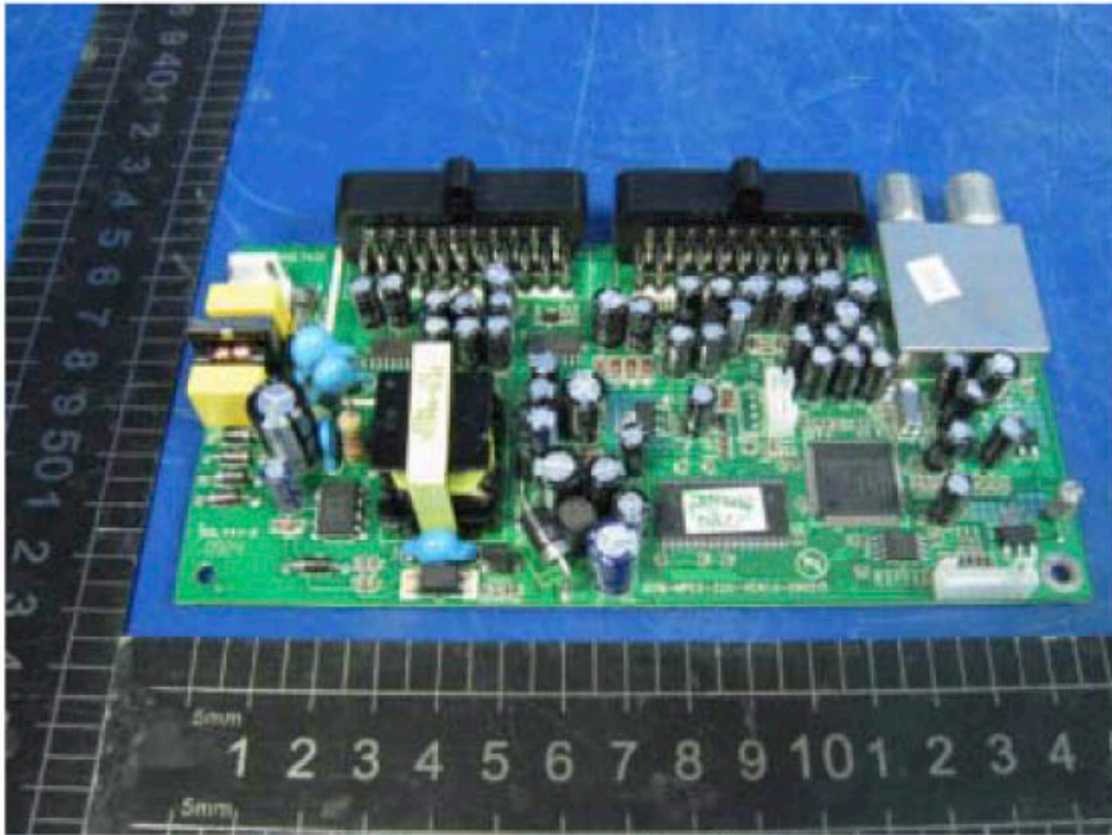
Photo 5 Power supply and function board
