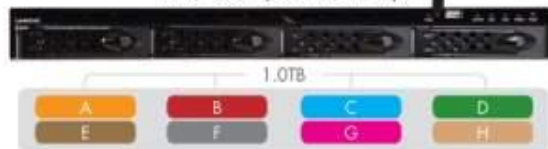
RAID 0 Striped No Parity
