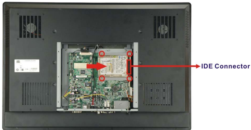
Figure 2-5: IDE HDD Installation
