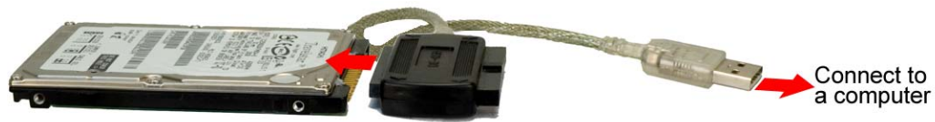
Figure 2-1: Format the HDD via IDE-USB Cable
