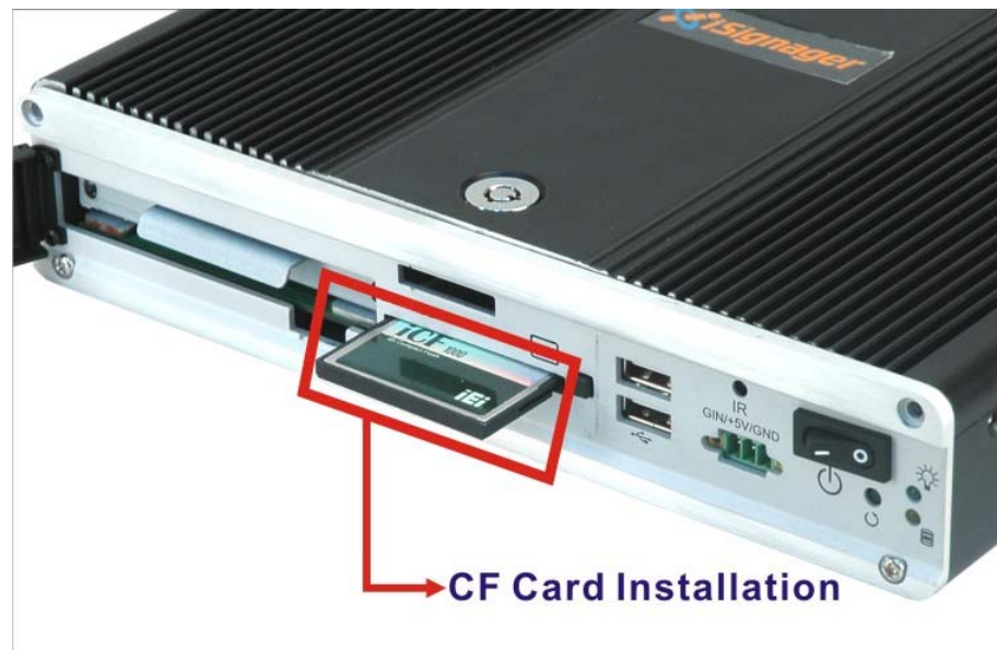
Figure 2-1: CF Card Location (Front Panel)
