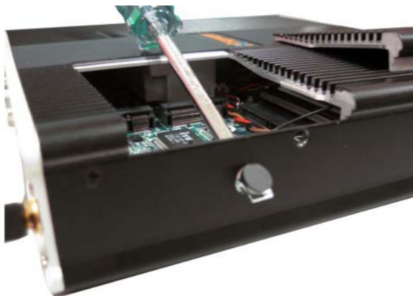
Figure 2-6: Open Antenna Connector Hole
