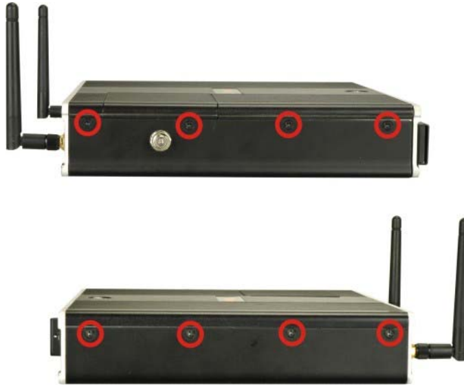
Figure 3-1: Top Cover Retention Screws (Side Panels)
