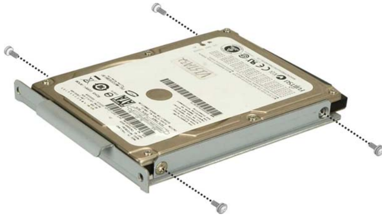
Figure 3-5: HDD Retention Screws
