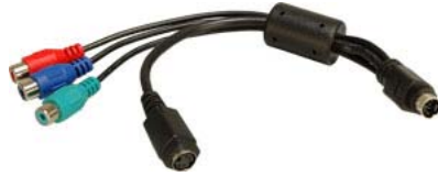
Figure 2-13: TV-out to Component Video/S-Video Cable
