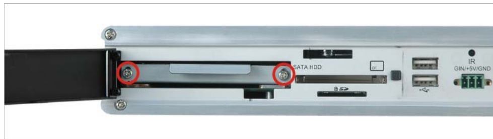
Figure 3-4: HDD Bracket Retention Screws
