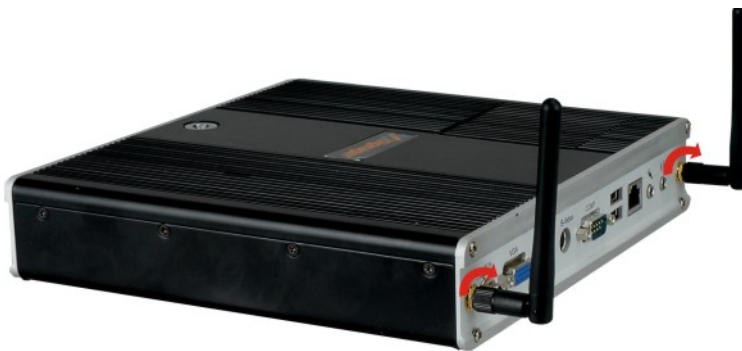
Figure 2-4: Wireless Antenna Installation
