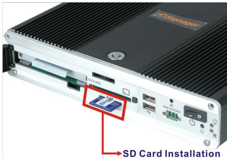
Figure 2-2: SD Card Location (Front Panel)
