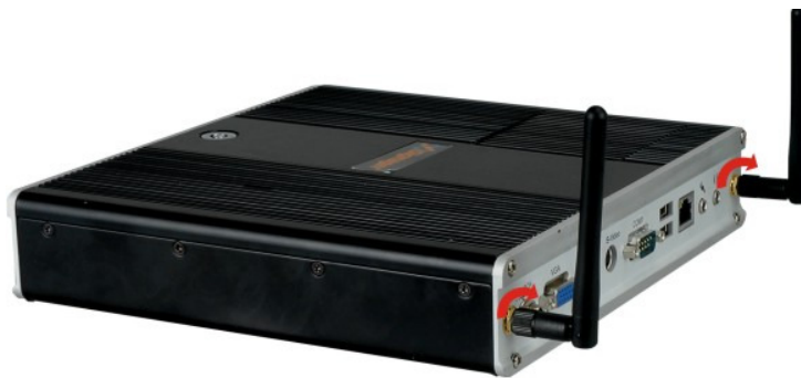
Figure 2-4: Wireless Antenna Installation
