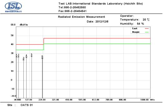
Condition : CISPR22 ClassA 10M Radiation Polarization: Vertical
