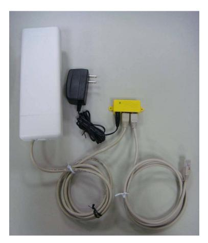
Notes: Use **Reset button** on POE injector. Push continually the reset button of POE injector about  $5 \sim 10$  seconds to reset the configuration parameters to factory defaults.
