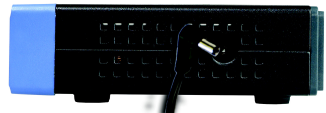
Figure 3-3: Connecting to the Power Port
