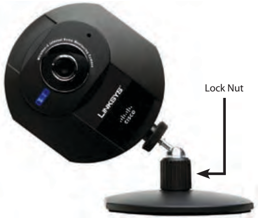
Camera Tilting Feature with Stand Option
