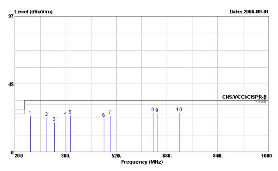
Site : OSO2-LK Condition : CNS/VCCI/CISPR-B 10m CBL6111C.2715.940924 VERTICAL EUT : NAS
