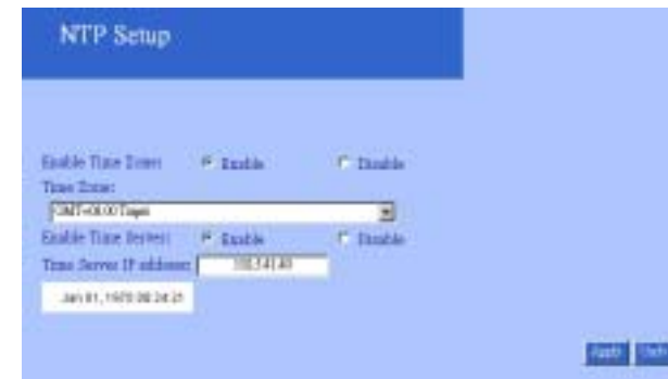
IP Camera Setting – NTP Time Service Setup
