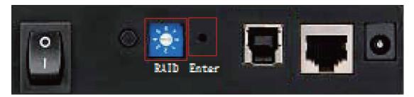
Notes: Please change to single mode before altering any modes of RAID disk array. Otherwise, it cannot be changed. Meanwhile, you should format the HDD by network mode after changing the setting of RAID disk array. After that, it can work in normal.
